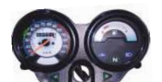
SPLNDR + with i3s - O/M Pricol Part No: 70854 OE Part No: P37100-AAE-1110
